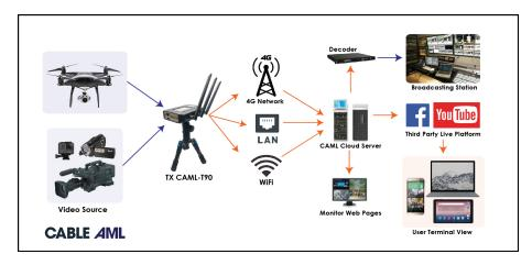
CAML-T90 is a real-time video transmission terminal based on multi link aggregation technology and H.265 coding technology. It is equipped with 3 built-in 4G modules and a USB expansion interface, Support for external modules: 4G/WiFi, supporting WiFi and cable network access.
